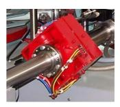
Figure 1. One of the quadrupole focus coil assemblies used in our linear accelerator
