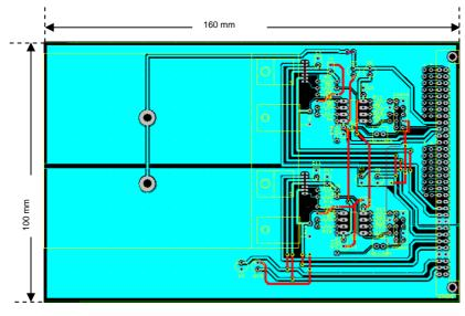
Figure 5a: The dual-sided printed circuit board layout of the constant current driver
