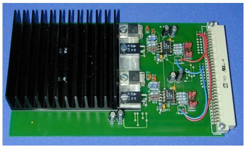
Figure 6. One of the completed boards housing two current source systems. The input currentsetting input voltage and the current monitor output voltage are 'linked' to Eurocard pins with the red/blue wire connections, as described in the text.
