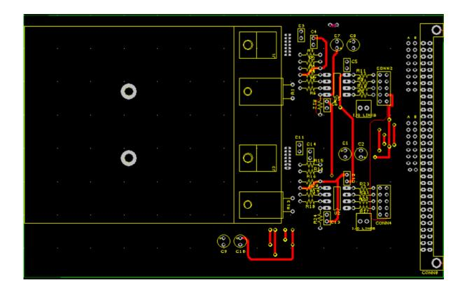
Figure 5b. The two layers of the double-sided board used in the constant current driver shown in Figure 3.
