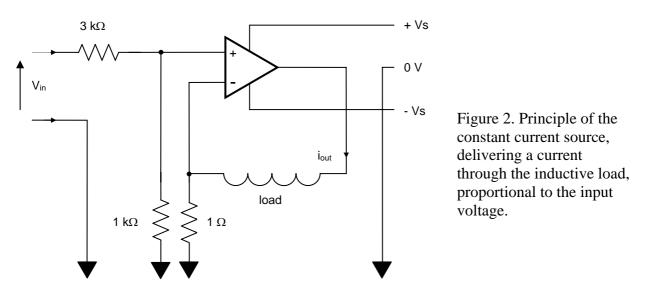
The circuit can deliver bipolar output currents, as determined by the polarity of the input voltage. As shown in Figure 3, this input voltage is derived from a differential amplifier, A1 or C1, arranged such that it can operate as a buffer or inverter, with or without a DC offset, depending on the links inserted at A1's (or C1's) input. The output current can be monitored by sensing the voltage across the 1  $\Omega$  current sensing resistor, appropriately amplified by opamps A2 and C2.
