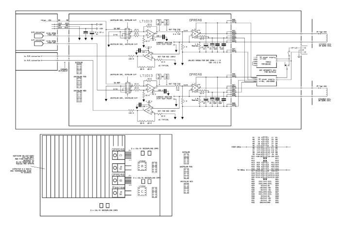
Figure 3. Circuit diagram of the constant current power supply board, arranged to house two identical circuits.
