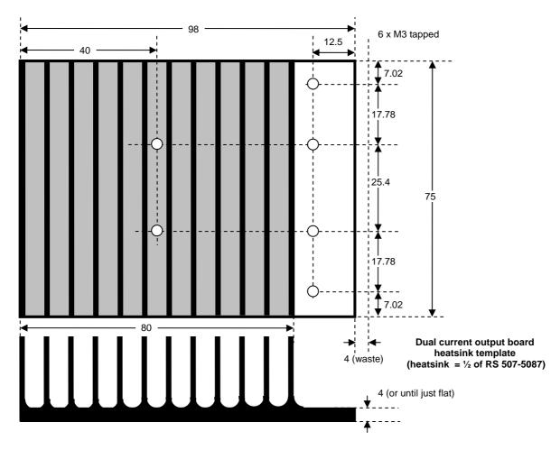
Figure 4. Dimensions of the 'cut-down' heatsink used in the constant current power supply board
